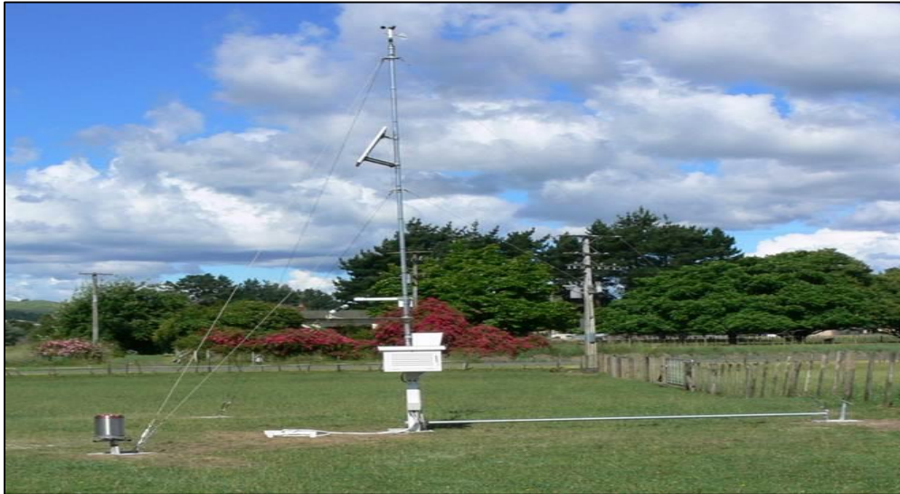
Automated Weather Station for 5 remote outer islands
